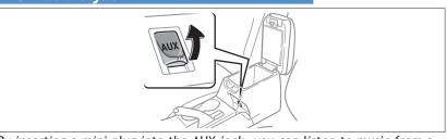
By inserting a mini plug into the AUX jack, you can listen to music from a portable audio device through the vehicle's speaker system while in AUX mode. If you do not have a SCION genuine audio system, you will not be able to use the AUX jack.
